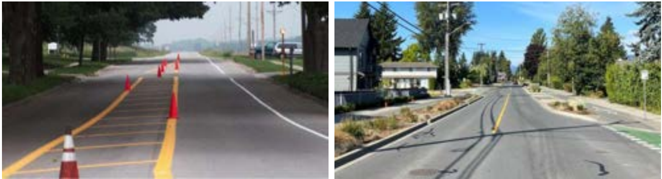
Figure 14. Sample Application of Lane Narrowing 22, 23
