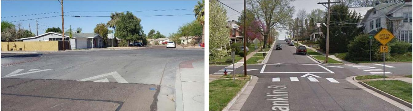
Figure 11. Sample Application of Raised Intersection<sup>16,17</sup>
