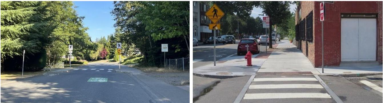
Figure 10. Sample Application of Raised Crosswalk<sup>14, 15</sup>
