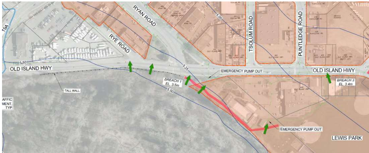
Figure 6-27: Location of AquaDam (thick red line) and Tall Wall (grey bars) near Lewis Park and along Old Island Highway (see Figure 6-37 for complete map) (Credit: McElhanney, 2022).
