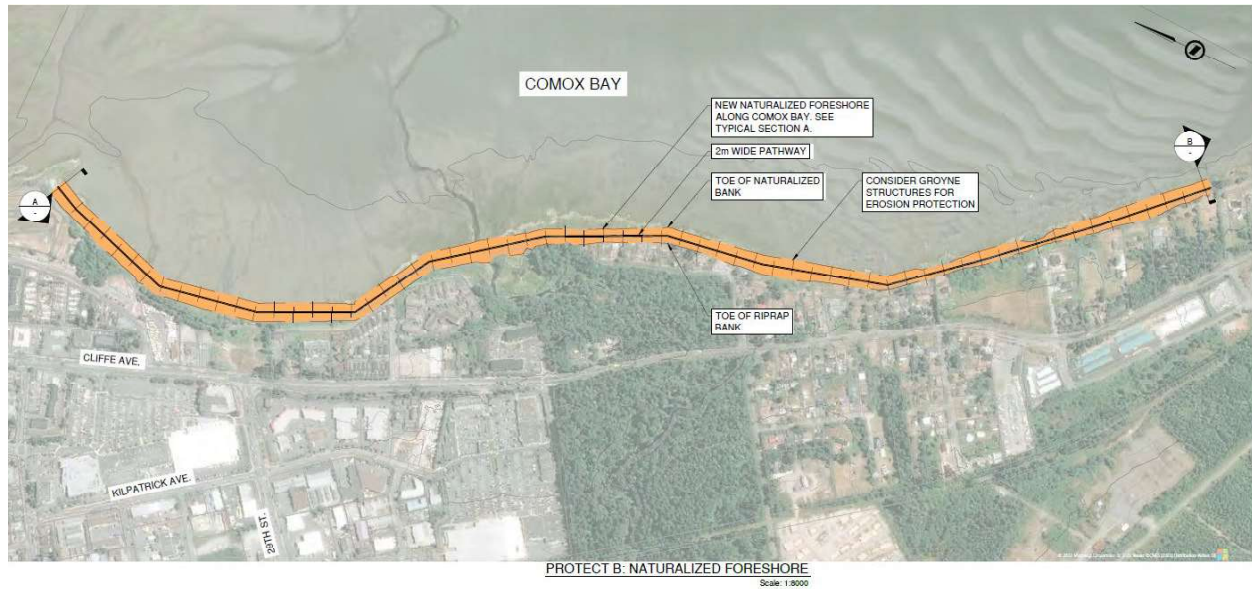
Figure 7-6: Conceptual drawing of proposed naturalized foreshore along coast (Credit: Water Street Engineering).
