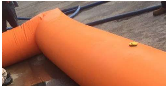
Figure 6-28: Tiger Dam. Credit: U.S. Flood Control.
