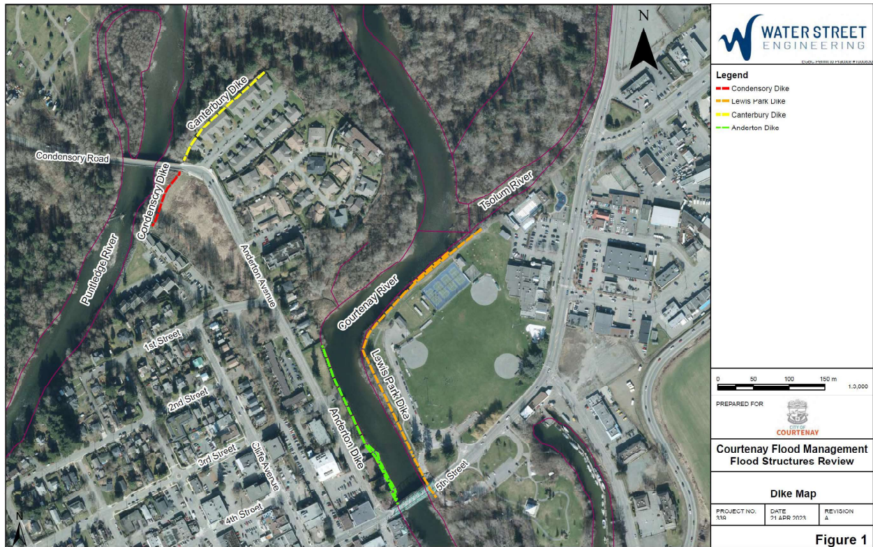
Figure 6-15: Dike Map (Credit: Water Street Engineering).
