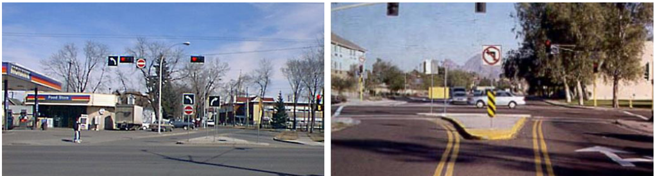
Figure 21. Sample Application of Intersection Channelization 32, 33
