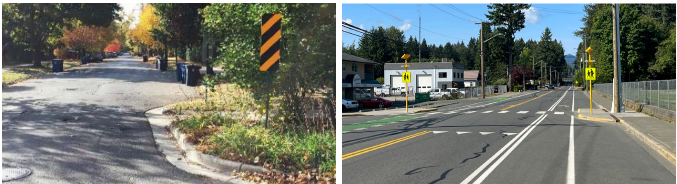
Figure 12. Sample Application of Curb Bulge 18, 19
