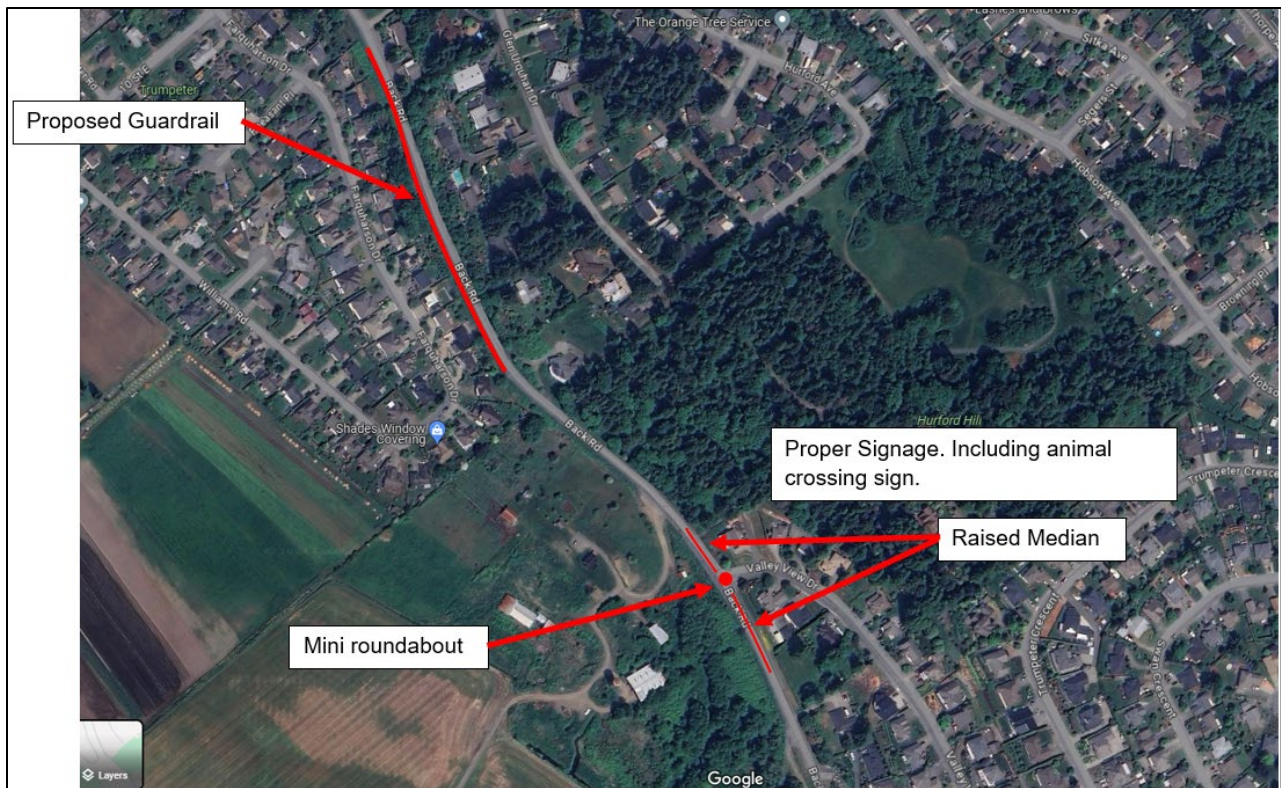
Figure 7: Conceptual Layout of the Proposed Traffic Calming Measures
